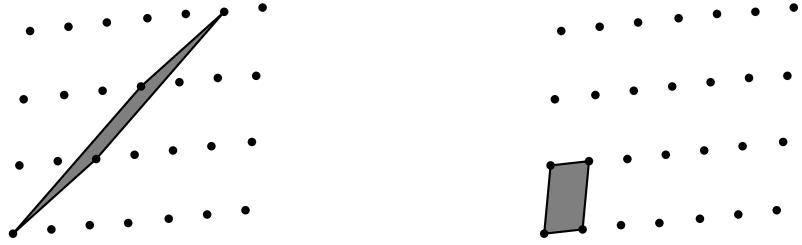
**Fig. 1.** A lattice and two of its bases represented by the parallelogram they span. The first basis is skew, the second one is minimal (reduced).
