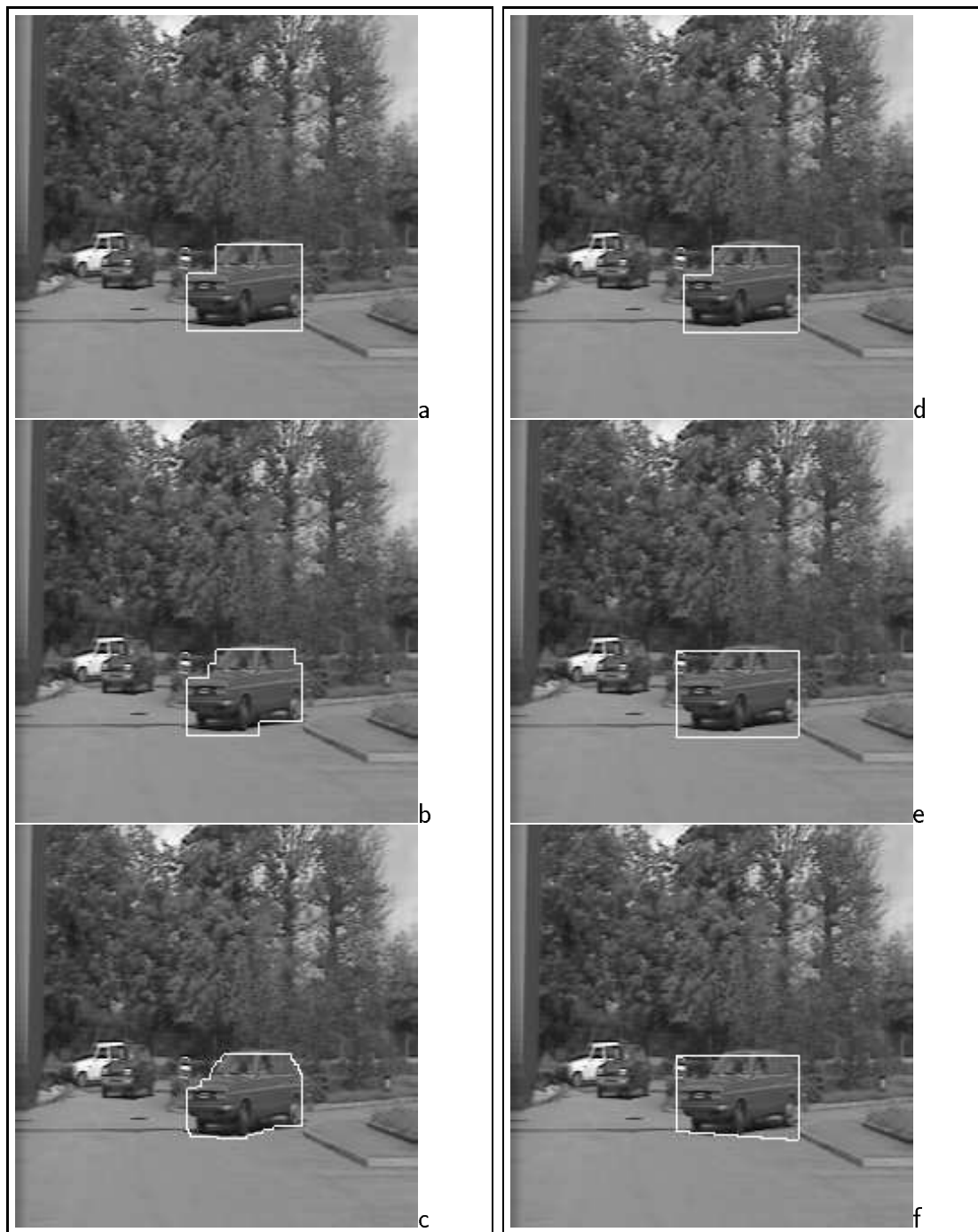
Figure 15: Single object motion segmentation on Parking lot: (a-b-c) with an unconstrained closed curve at grid levels 4,2 and 0 (d-e-f) with a convex quadrilateral at grid levels 4,2 and 0.
