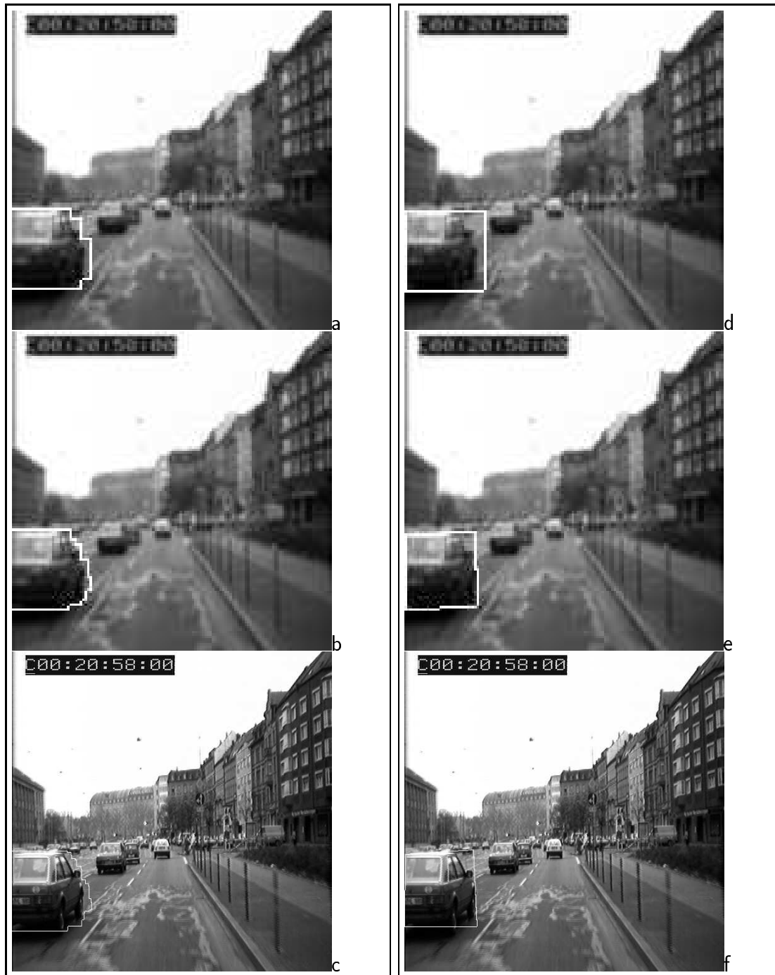
Figure 16: Single object motion segmentation on Street: (a-b-c) with an unconstrained closed curve , in \Omega^{2,2} , \Omega^2 and \Omega (d-e-f) with a convex quadrilateral in \Omega^{2,2} , \Omega^2 and \Omega .
