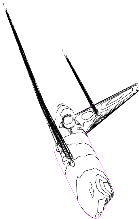
Figure 10: Research by shape optimization of a more uniform pressure on a Falcon aircraft : iso-gradients contours on the body.
