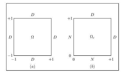
Figure 2. (a). The Domain  $\Omega$  with Dirichlet Boundary Conditions (b). The Domain  $\Omega_r$  with Neumann and Dirichlet Boundary Conditions
