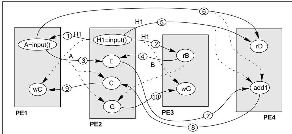
FIGURE 10. Partitioning and processor communications after Springplay scheduling
