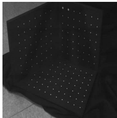
Figure 3: The calibration grid, this grid is composed of retro-reflective targets.
