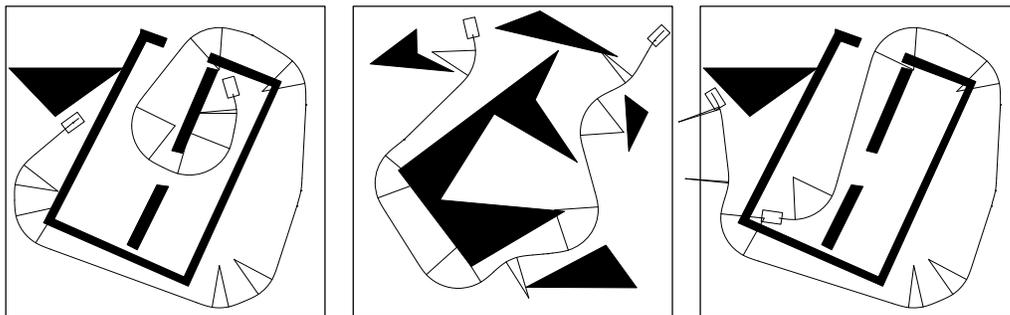
Figure 4: Examples of continuous curvature paths.
