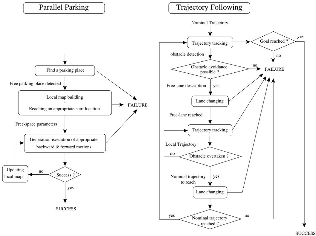
Figure 6: The “parallel parking” and “trajectory following” SBMs.
