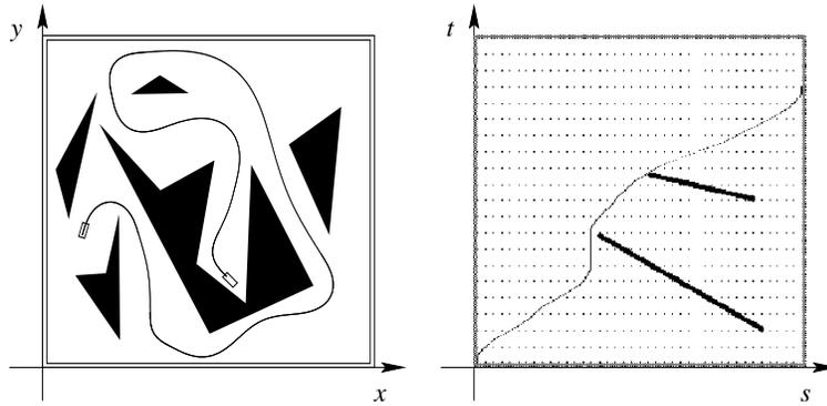
Figure 3: (a) Path planning and (b) velocity planning.
