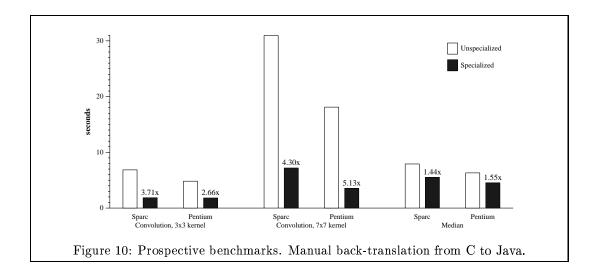
The performance of the specialized code is significantly better than that of the generic, unspecialized code. We have tested the automatically specialized code using the Harissa environment. Experiments were conducted both on a Sun workstation (300MHz UltraSparc) and on a Dell PC (200MHz Pentium Pro). The results, including both the execution time and the speedup of the specialized code, are shown in Figure 9.
