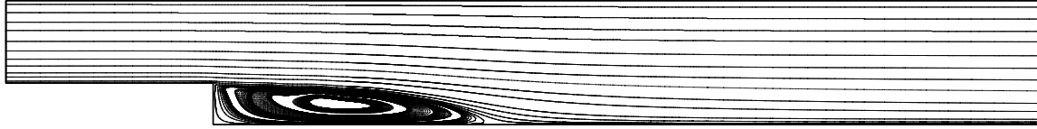
Figure 41: Streamlines in the plane z = 0. , Re = 44000.
