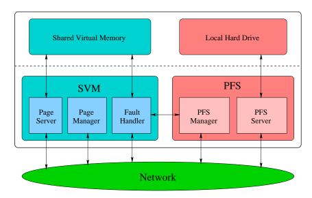
Figure 1: Software architecture of the prototype
