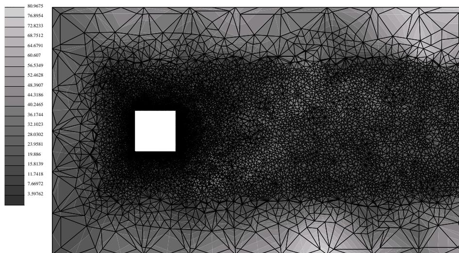
Figure 8: Ratio between the SGS viscosity and the gas viscosity;  $C_s = 0.1$ ,  $\Delta_{\epsilon q}$  defined in Eq. (73).
