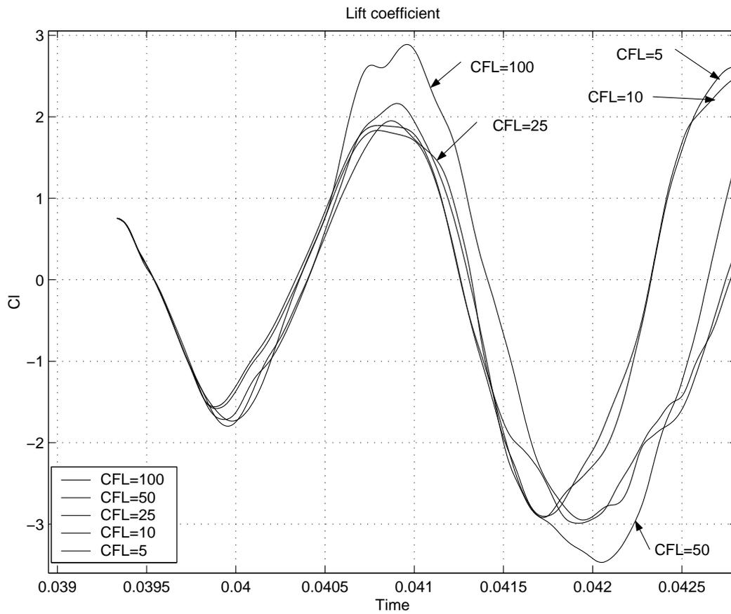
Figure 10: Lift curves obtained with different CFL numbers.
