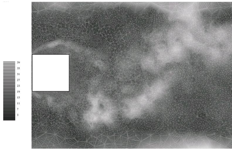
Figure 7: Ratio between the SGS viscosity and the gas viscosity;  $C_s = 0.1$ ,  $\Delta_{\epsilon q}$  defined in Eq. (73).
