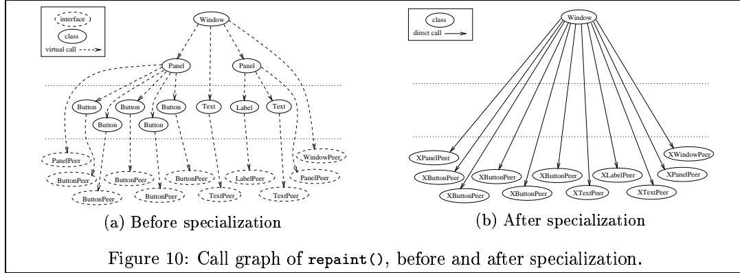
Figure 10: Call graph of `repaint()`, before and after specialization.
