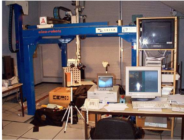
Figure 11: Experimental setup at IRISA-INRIA Rennes: six degrees of freedom cartesian robot with a camera mounted on the end-effector.
