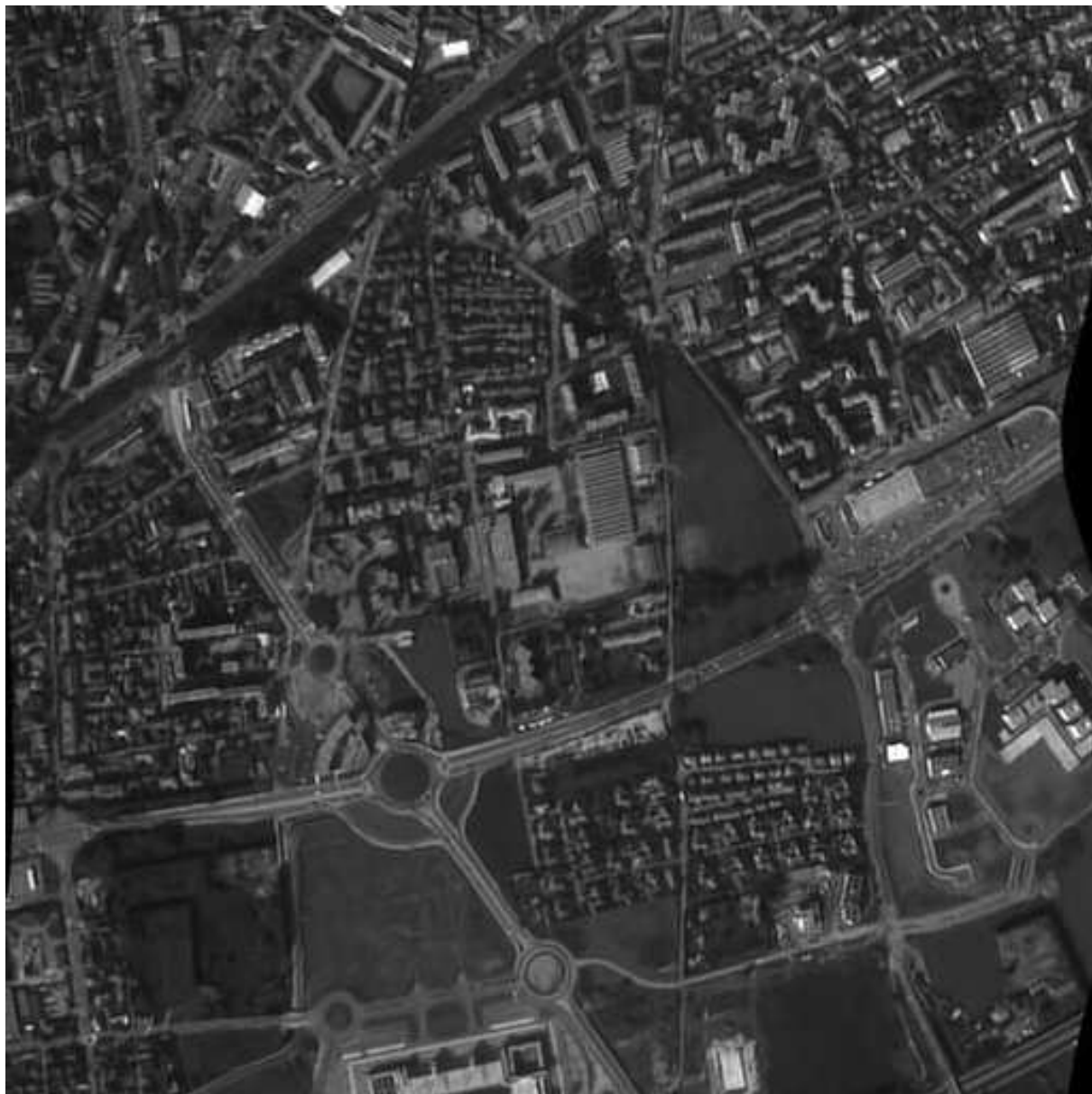
Figure 4.5: Image of Fig. 4.1 deconvolved with the fast version of Algo. 3.4.2 (COWPATH 2) - SNR=22.1 dB
