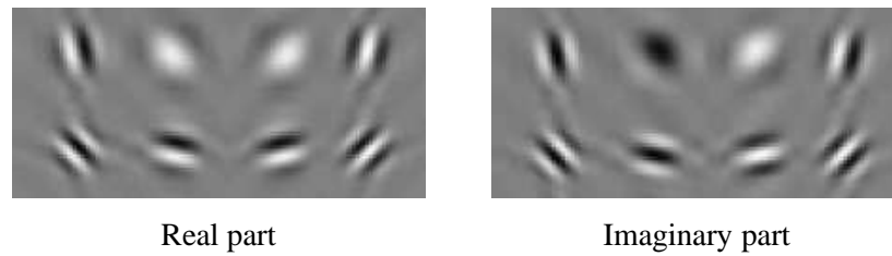
Figure 3.8: Impulse response of the complex wavelet transform at level 4, showing the ability to separate 6 directions
