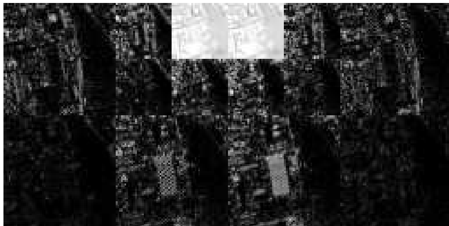
Figure 3.10: Magnitude of the complex wavelet transform of the original image of Fig. 1.1
