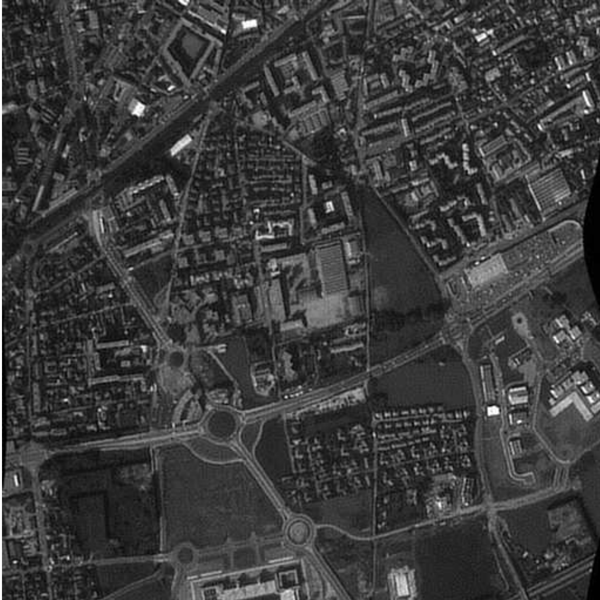
Figure 4.10: Image of Fig. 4.1 deconvolved with quadratic regularization (Tikhonov) and optimal hyperparameter b = 0.0005 - SNR=19.6 dB
