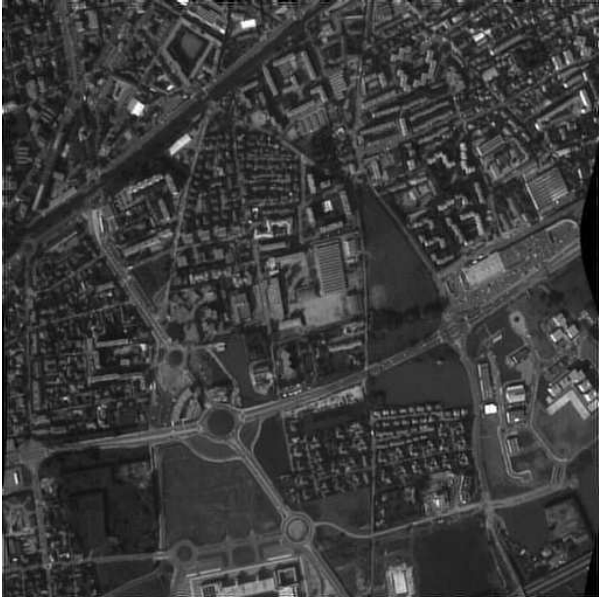
Figure 4.10: Image of Fig. 4.2 deconvolved by a real wavelet packet thresholding algorithm [25] - ASNR=24.6 dB
