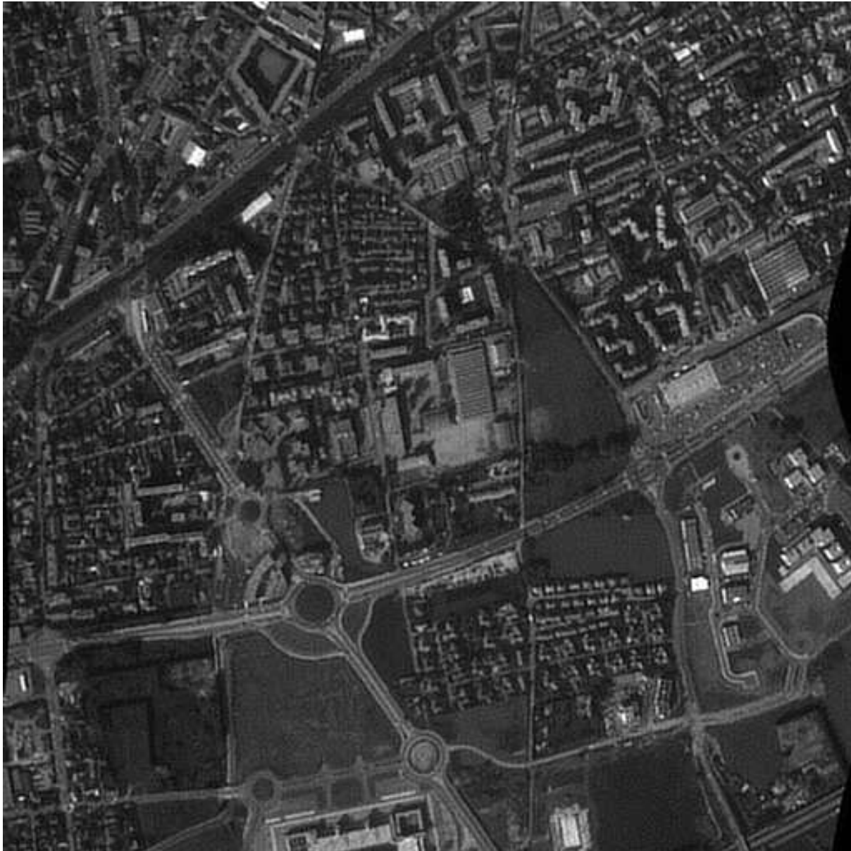
Figure 4.8: Image of Fig. 4.2 deconvolved with quadratic regularization (Tikhonov) and optimal hyperparameter b = 0.0005 - ASNR=19.7 dB
