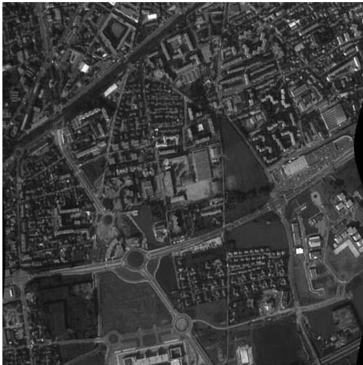
Figure 4.9: Image of Fig. 4.2 deconvolved with RHEA algorithm - ASNR=24.5 dB
