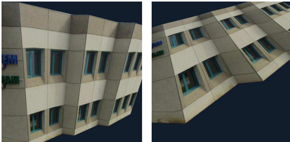
Figure 21: Textured rendering of the recovered projective model for the Game System stereo image pair from different points of view.
