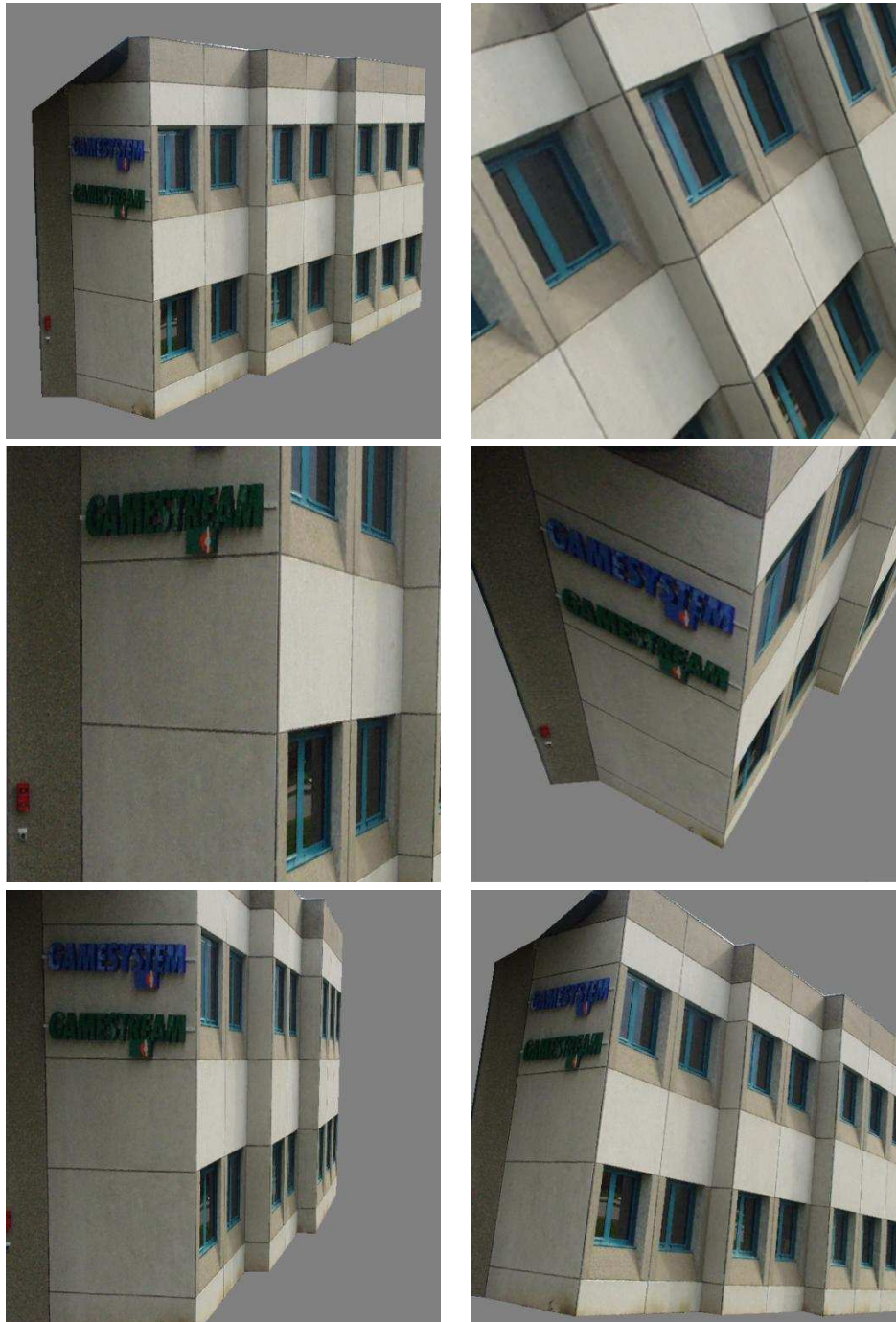
Figure 22: Textured rendering of the recovered metric model for the Game System stereo image pair from different points of view.
