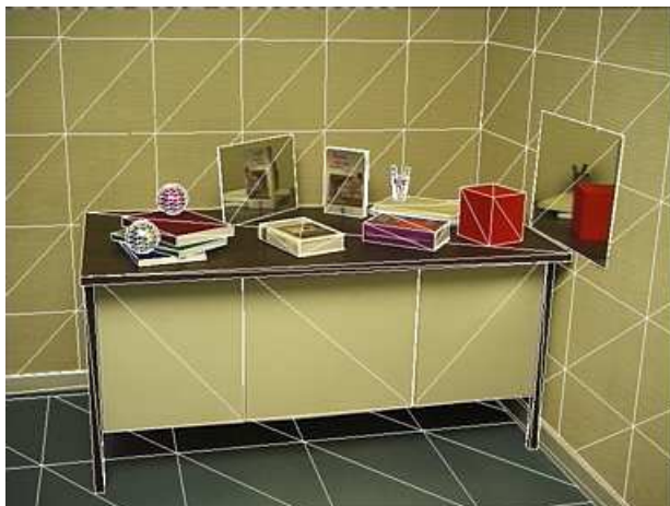
Figure 2: Example of a real image with the superposition of its 3D reconstructed geometrical model (in white)
