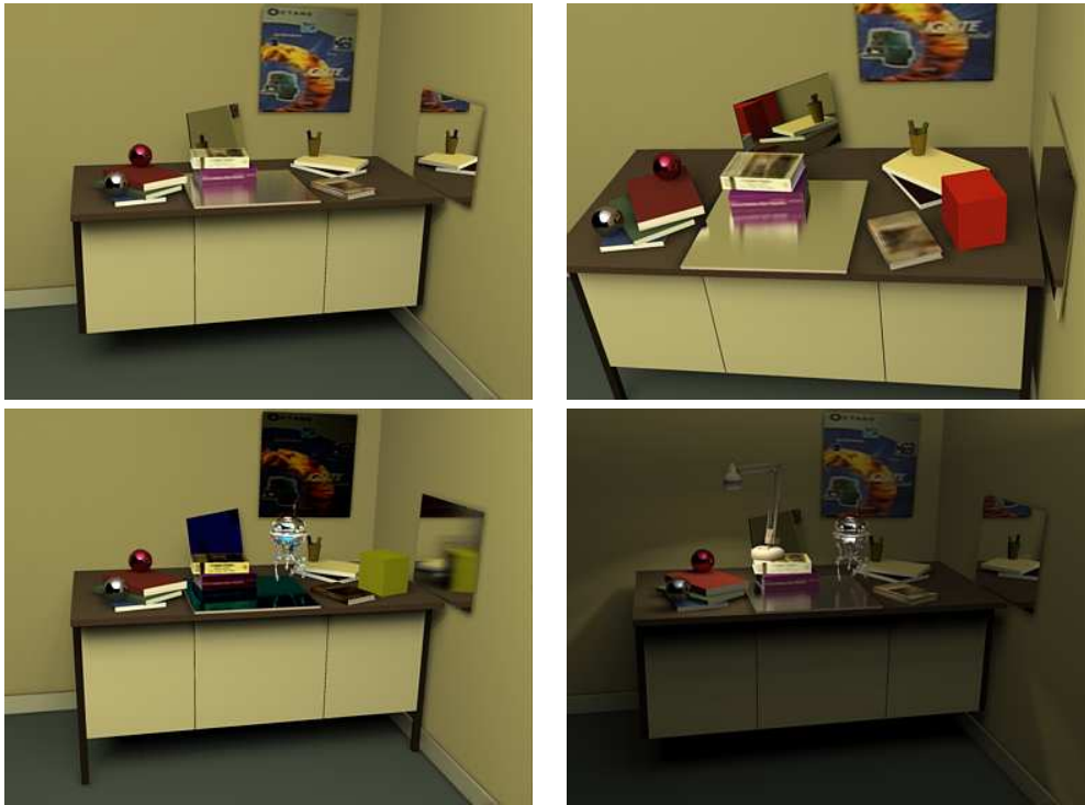
Figure 15: Examples of several augmented reality applications. All these new images were rendered using our global illumination software Phoenix , which first recovered the surface reflectances from the bottom left image of figure 14. The top left image shows the original scene removing some objects (the feet of the desk and the red cube). Note that the right mirror has taken into account the modification. The right top image shows the original scene rendered under a novel viewpoint. The bottom left image shows the scene with modified photometric properties, and the addition of an object (a small robot). The bottom right image presents the scene under novel illumination conditions with the addition and deletion of objects.
