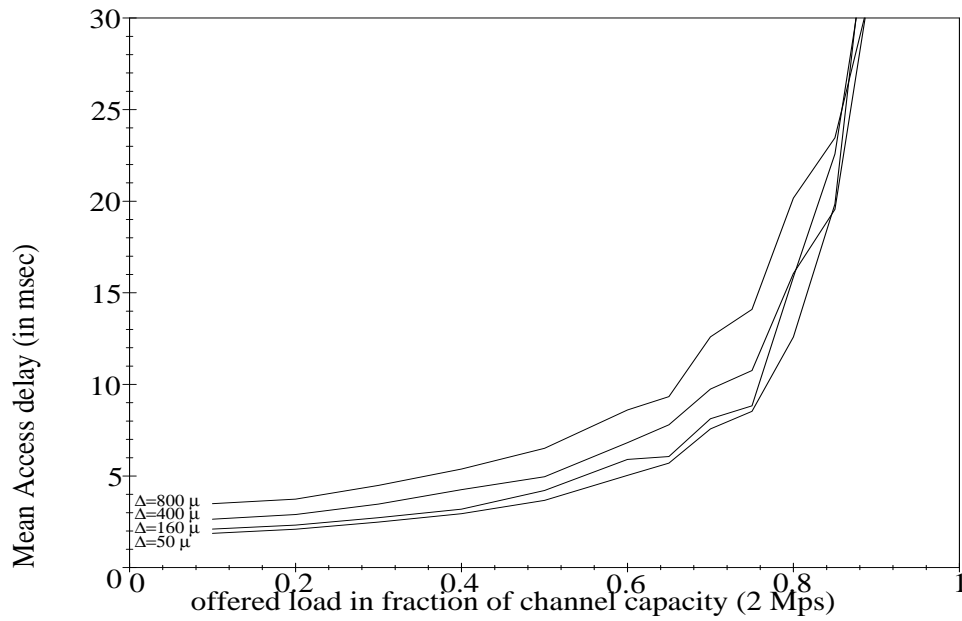
Figure 17: Mean access delay versus offered load, with parallelized 4-ary tree algorithm with N = 50 active users and varying feedback times. Case 1, Feedback time \Delta = 50 \mu\text{sec} (5 km), \Delta = 160 \mu\text{sec} (16 km), \Delta = 400 \mu\text{sec} (40 km), \Delta = 800 \mu\text{sec} (80km). Magnified part of previous figure.
