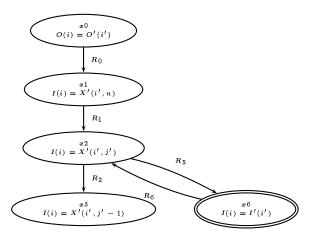
The automaton is constructed on demand from the initial state O[i] = O'[i'], expressing the fact that the two SAREs have the same output. For instance, edge R0 is an application of "Computation" both on the left and right of the initial state. Edges R1 and R6 are generalizations. State x3 is a success state, and there are no failure states. Edge names also stand for the corresponding firing relation. For instance, R6 is:
