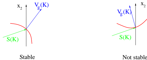
Figure 14: Two different configurations. Left: the slowness vector \vec{S} and the group velocity V_g are oriented in the same way with respect to the Ox_2 axis. Right: \vec{S} and V_g are not oriented in the same way with respect to the Ox_2 axis.
