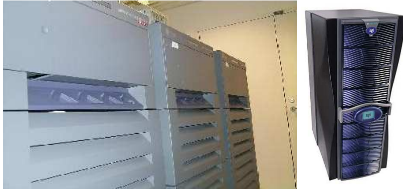
Figure 2: Left: Wildfire Cluster with scalable memory, architecture built on SUN E5k and E6k chassis, 36 250MHz UltraSPARC-II CPUs and 9GB RAM (source: [Kik00a]); Right: SGI Origin 3400, architecture built on 32-processor shared-memory system and 64GB RAM under IRIX 6.5 (source: http://www.sgi.fr/servers/ ).
