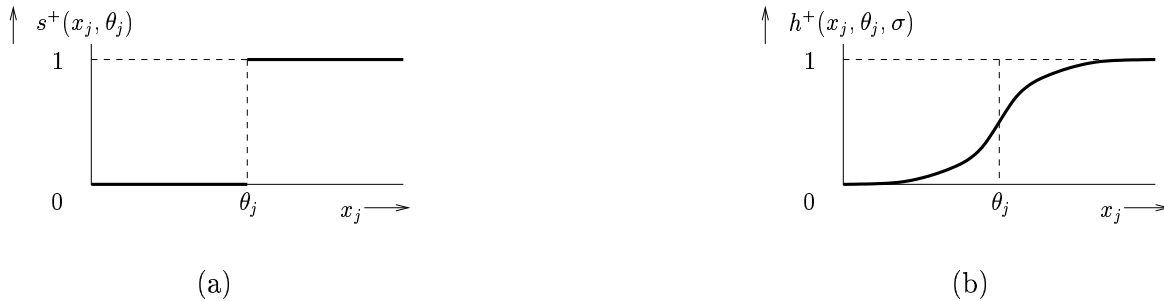
Figure 7: Different threshold functions: (a) step function s^+(x_j, \theta_j) and (b) sigmoid function h^+(x_j, \theta_j, \sigma) . The sigmoid function approaches the step function as \sigma \rightarrow \infty .
