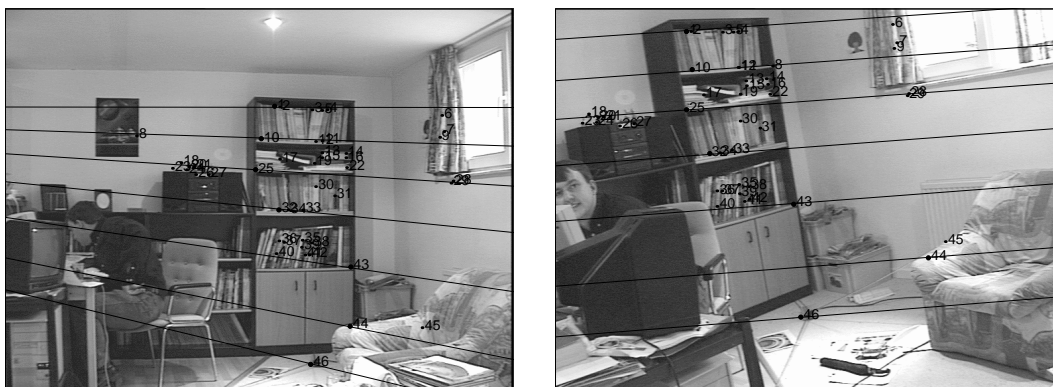
Figure 12: This figure shows the epipolar geometry as computed with the matching and estimation method described in this report. Notice the large discrepancy in the viewpoints associated with the two images. The matcher seems to give advantage to collections of coplanar points.
