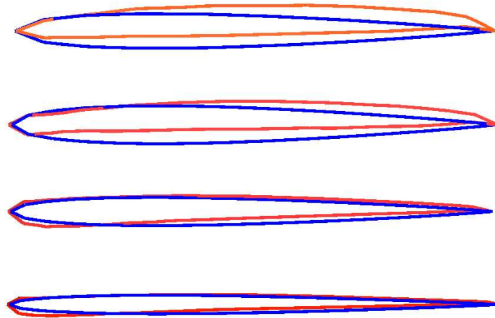
Figure 16: Isolated wings of the Supersonic Business Jet. Optimization Strategy II. Shape optimization shown at the four wing sections. From top to bottom: Sections A, B, C and D. In blue, the original shape.
