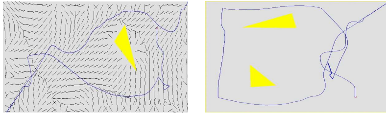
Figure 11: Showing how the same mechanism is used in the absence of any goal. As expected, a wandering behavior is generated. In the left view, the potential generated during the trajectory is shown, the geometry of the field is clearly induced by the geometry of the obstacles. In the right view, it is made visible that some parts of trajectory corresponds are straight and some are bended with several walk around the same position. These two qualitative effects are directly related to the evolution of the potential.
