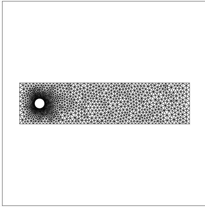
Figure 18: Computational mesh around the cylinder
