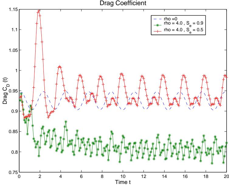
Figure 21: Drag evolution for different control parameters
