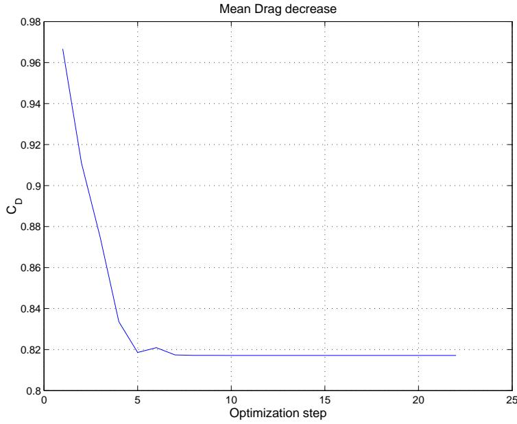
Figure 27: Mean drag evolution- 3 harmonics case
