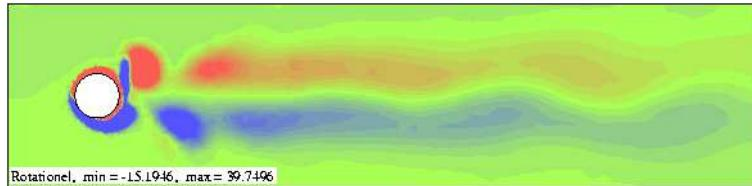
Figure 24: Vortex shedding in the optimal controlled case
