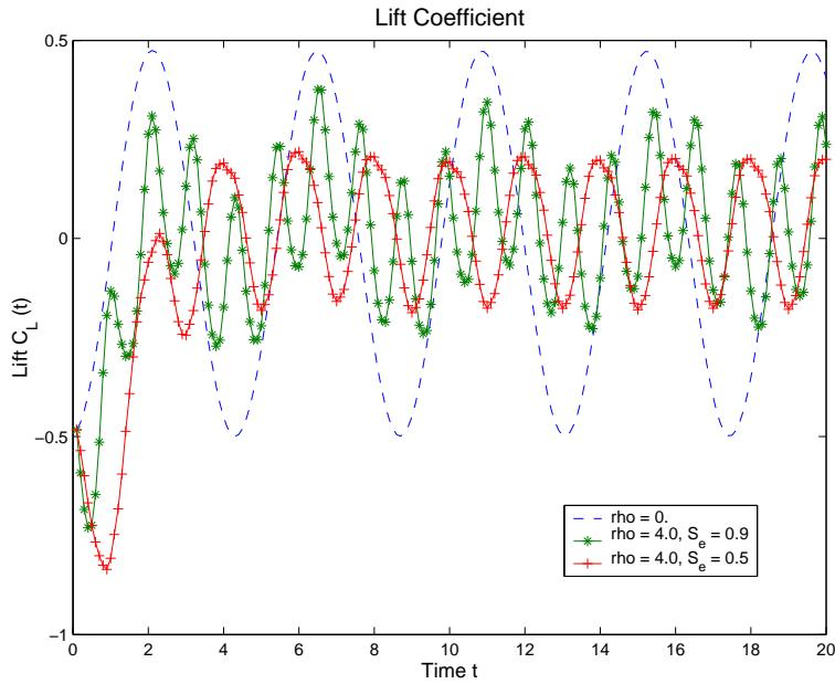
Figure 22: Lift evolution for different control parameters
