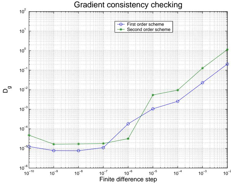
Figure 39: First and second order Lagrange-Galerkin scheme applied to the moving R4 profile - Gradient test
