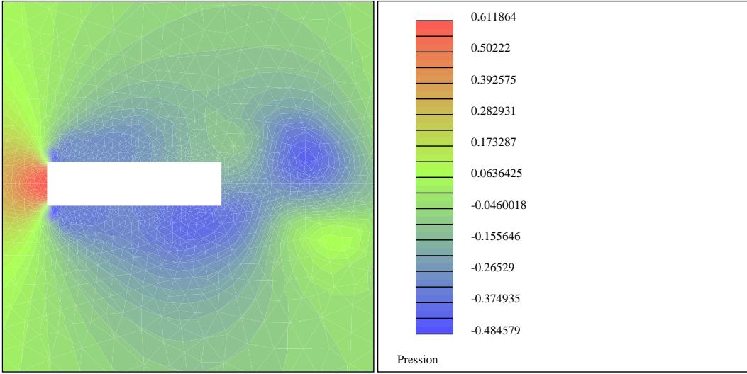
Figure 30: Pressure profile for the R4 rectangular cylinder
