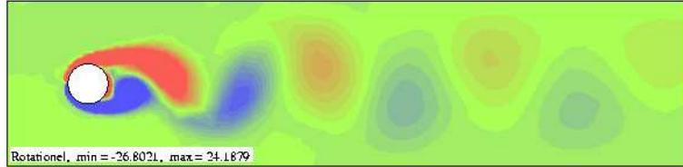
Figure 23: Vortex shedding in the uncontrolled case
