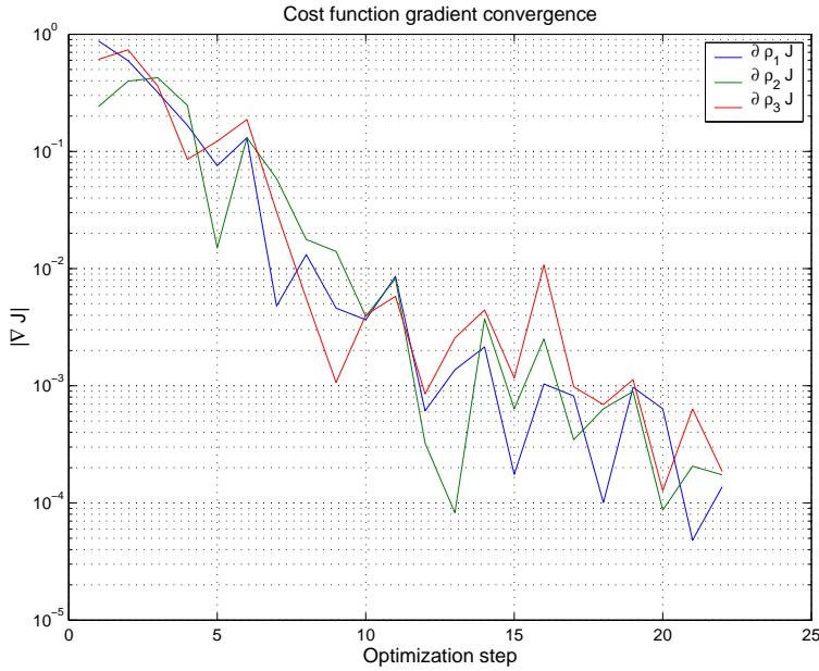
Figure 28: Cost function gradient decrease - 3 harmonics case
