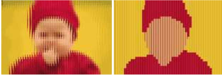
Figure 2: image of LDQC's (left) and image of LDQC prototypes after clustering (right). These two images are created to visualization all the LDQC's in the image: each square neighborhood is replaced by the corresponding local color distribution drawn with color bars of width proportional to the quantized color population.
