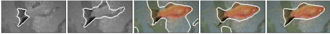
Figure 7: Benefits of using jointly colour and texture information. FROM LEFT TO RIGHT: (a) Grey value. (b) Grey value and texture. (c) Colour (RGB). (d) Colour (CIELAB). (e) Colour and texture.
