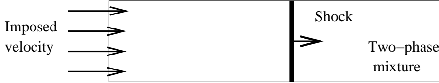
Figure 7: Schematic representation of the two-phase impact problem
