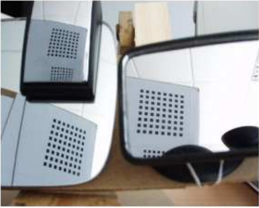
3 Mirror + pinhole camera (non-central scenario)
