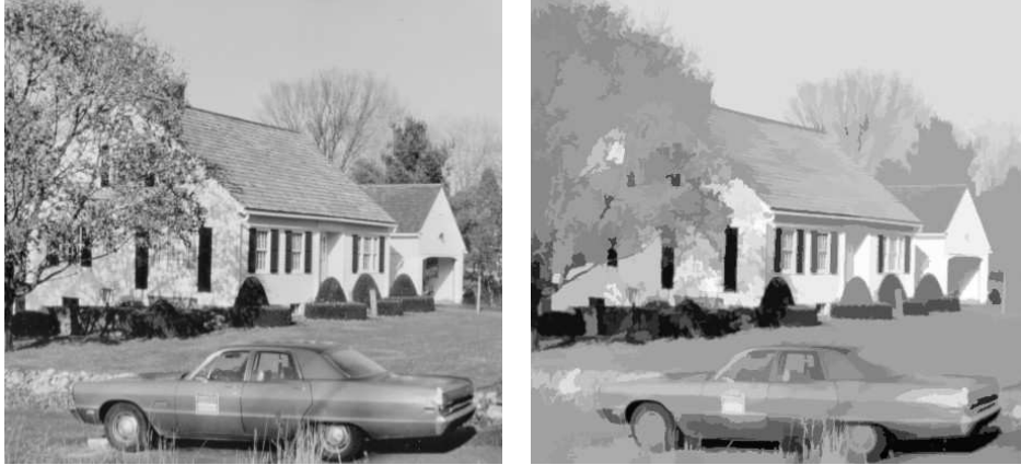
Figure 3: Original image on the left (99,829 level lines). Right: reconstruction from the 429 maximal meaningful boundaries. The gray level may not be really significant since, on edges, the maximal meaningful level line has an intermediate level between both sides of the edge. It would be more perceptually adequate to set the gray level to the brighter or darker meaningful level line. Nevertheless, for contrast independent shape recognition purposes, we do not use the grey level value, but only the geometry of level lines. The most important is that we preserved the main shapes, while removing the textures.
