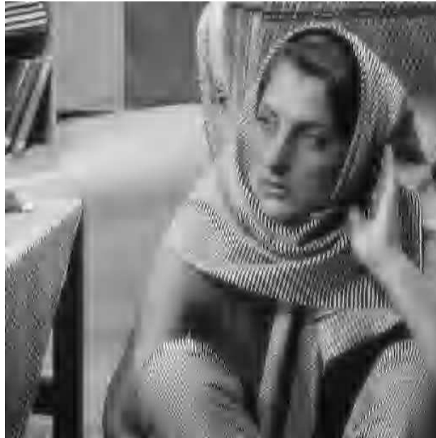
Figure 13: Compressed image with biorthogonal wavelets (BW) (20% of the coefficients)
