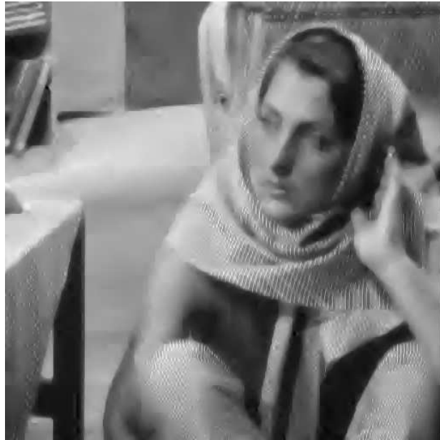
Figure 10: Compressed image with our method (UVEA) (10% of the coefficients for both the u and the v component)
