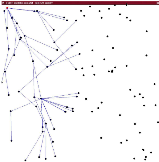
Figure 8: Routes of a node with signed messages
