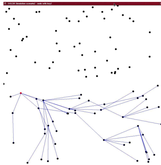
Figure 11: Routes of a node with second key
