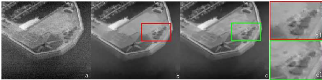
Figure 7: Infra-red sequence. (a) one image of the original sequence, (b) the corresponding image of the denoised sequence with the non-local filter applied with a patch of size 5 \times 5 and the bandwidth equal to four times the noise standard deviation, (c) denoised image with the proposed motion compensated filter, (b1) Cropped region of (b), (c1) Cropped region of (c).
