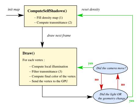
Figure 3: The rendering pipeline.
