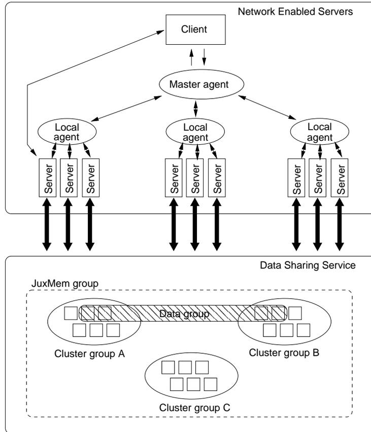
Figure 6: Overall architecture of the grid data-sharing service.
