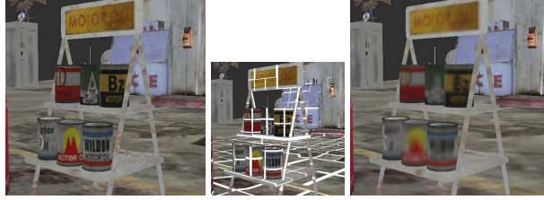
Figure 12: Two viewpoints rendered with 11 MB. Left picture is obtained with our system, right picture is obtained with a resized version of the texture. Details are preserved by our system.
