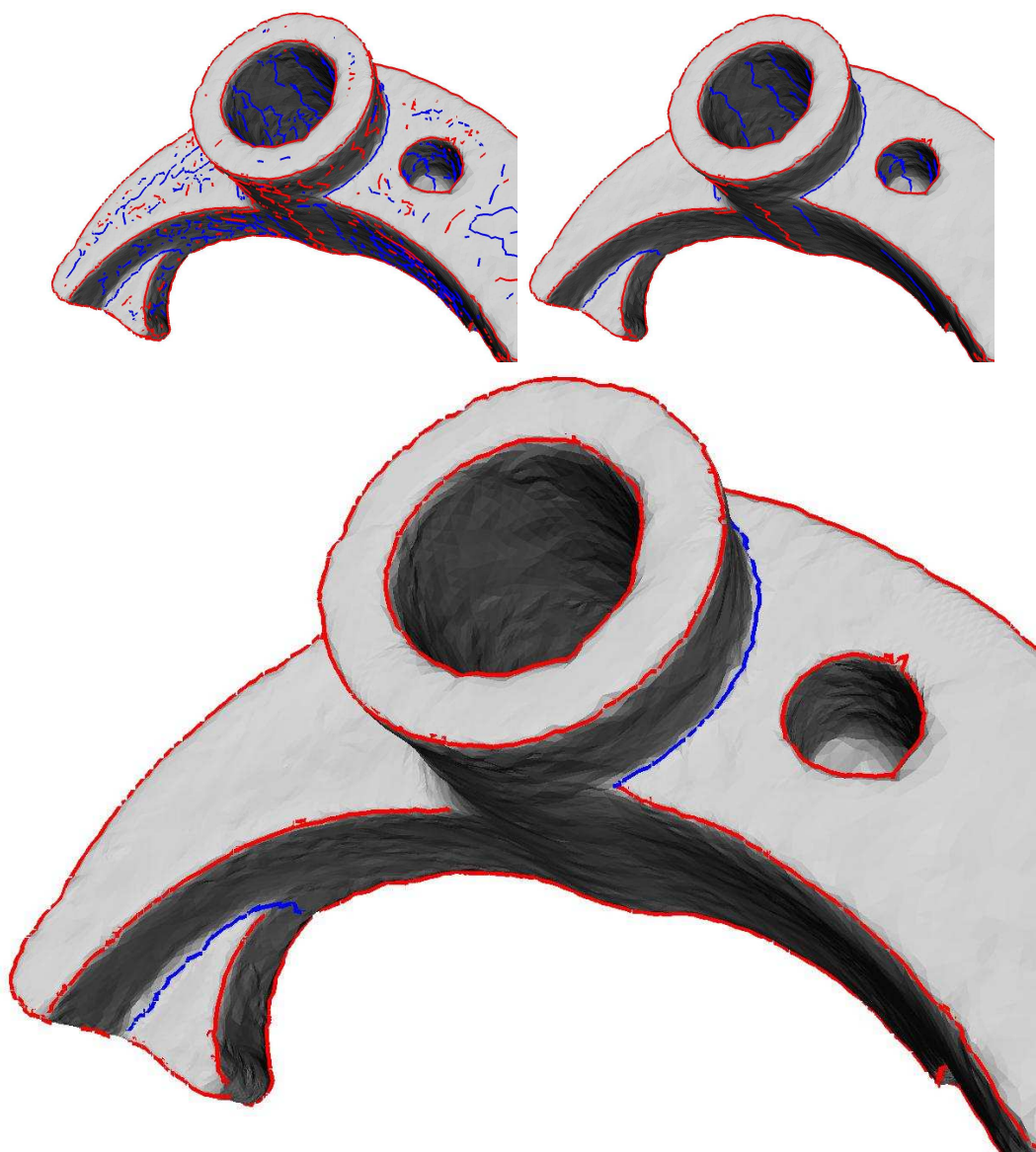
Figure 26: Mechanical part (37k pts): All crest lines, crests filtered with the strength and crests filtered with the sharpness. Notice that any point on a flat or cylindrical part lies on two ridges, so that the noise observed on the left two Figs. is unavoidable. It can however easily be filtered out using Observation 3.
