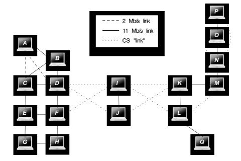
Figure 2: An ad hoc network presenting all performance issue configurations
