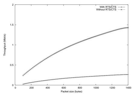
Figure 6: Throughput on a six-hops chain
