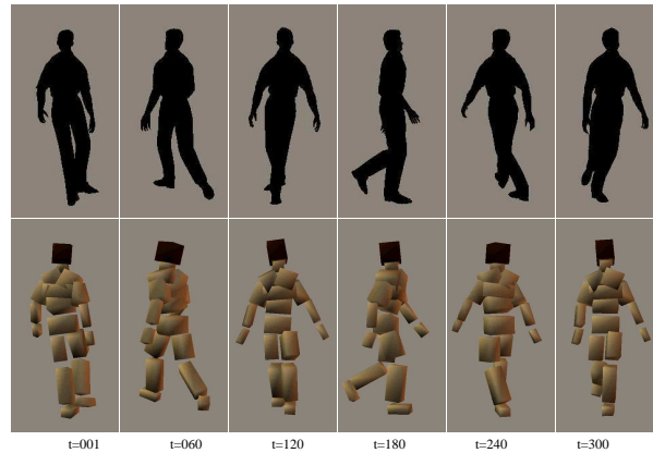
Figure 16: Sample pose reconstructions for the spiral walking sequence using the tracking method. This sequence was not included in the training data, and corresponds to figures 15(c) & (f). The reconstructions were computed with a Gaussian kernel RVM, using only 18% training examples. The average RMS estimation error per d.o.f. over the whole sequence is 4.1^\circ .
