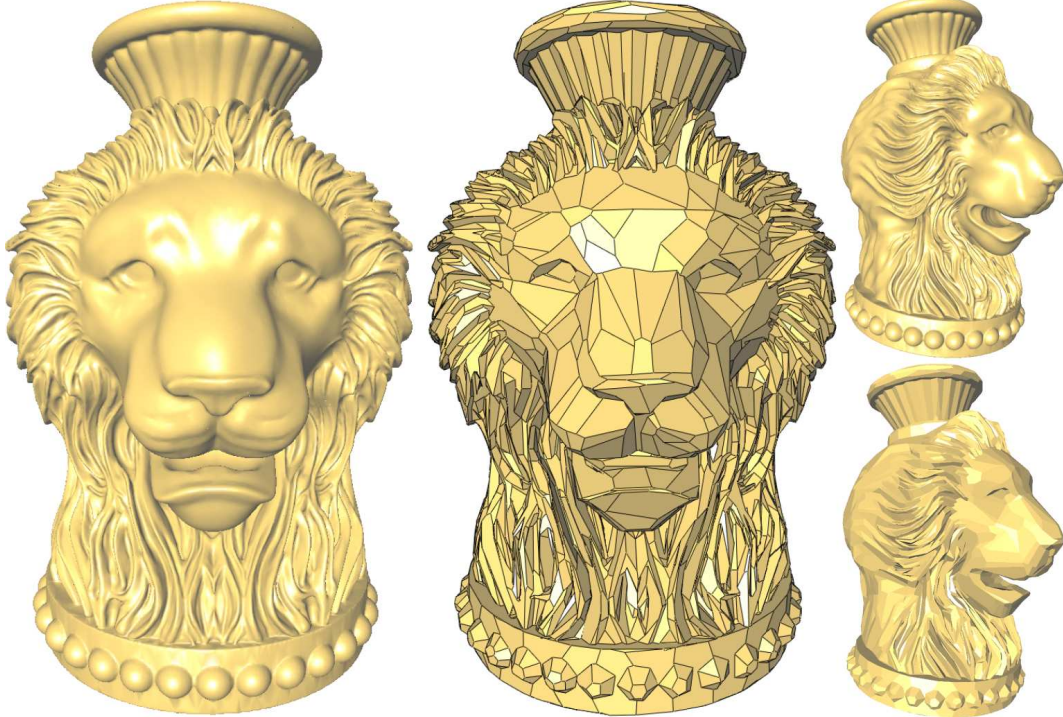
Figure 2: Lion-vase (400K-face model): Our shape approximation algorithm distributes mesh elements according to local surface complexity. (Right) Flat shaded comparison between original model and its 5K-polygonal \mathcal{L}^{2,1} -approximation (5 min, no user interaction); notice the good preservation of shape and highlights.
