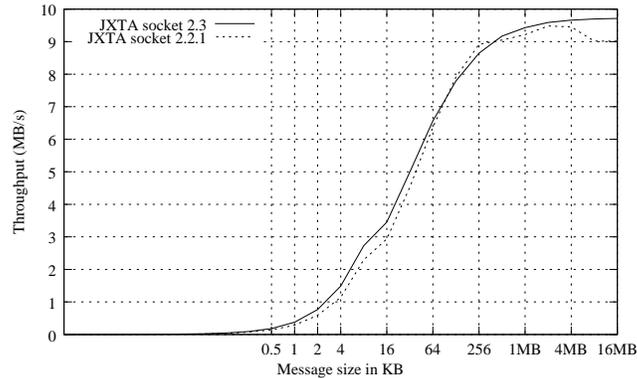
Figure 4: JXTA socket throughput using JXTA 2.2.1 and 2.3.
