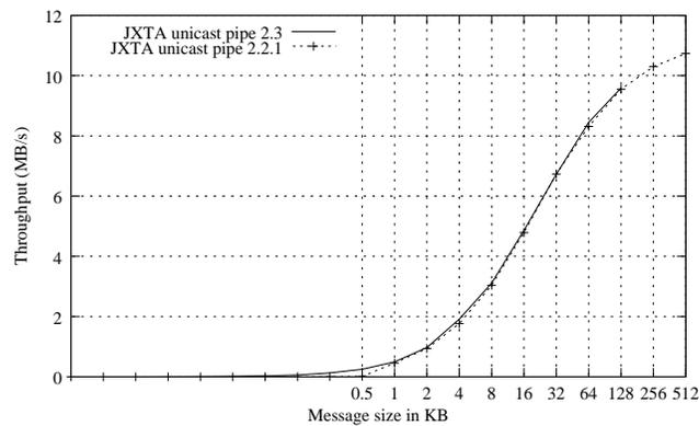
Figure 3: Unicast pipe throughput using JXTA 2.2.1 and 2.3.
