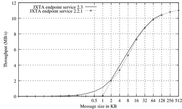
Figure 2: Endpoint service throughput using JXTA 2.2.1 and 2.3.
