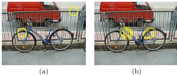
Fig. 1: Illustration of feature selection. (a) Two similar regions which cannot be used in a purely appearance based system to distinguish between the bicycle and the background. (b) The most discriminative features of the bicycle determined by our method.
