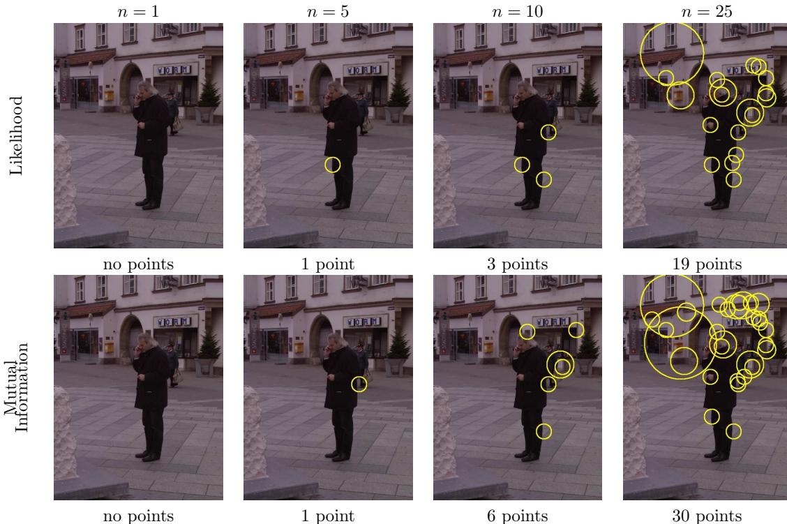
Fig. 8: Feature selection results with increasing n on a sample from the people database. This is one of the most challenging databases as the appearance of the people is very variable. In this case likelihood and mutual information focused on different part classifiers , there were no “very special” or “very general” clusters.
