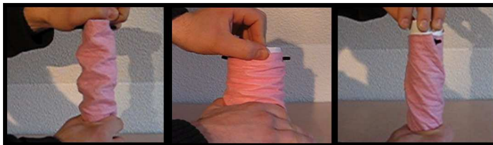
Figure 1: Buckling behaviour of real cylindrical panels of fabric. Diamond shape patterns (left and middle) appear under axial compression, since the surface maintains a zero Gaussian curvature everywhere during deformation. Twist patterns (right) made of parallel oblique wrinkles appear when one end of the panel is twisted.
