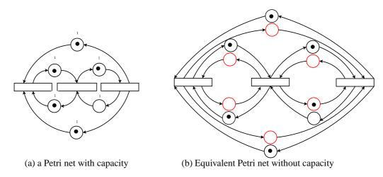
Figure 3: From a Petri net with capacity (a) to an other Petri net without capacity but with the same behaviour (b)
