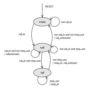
Figure 6: Relay Station FSM
