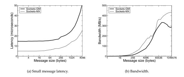
Figure 8: SOCKETS-MX and SOCKETS-GM performance comparison.
