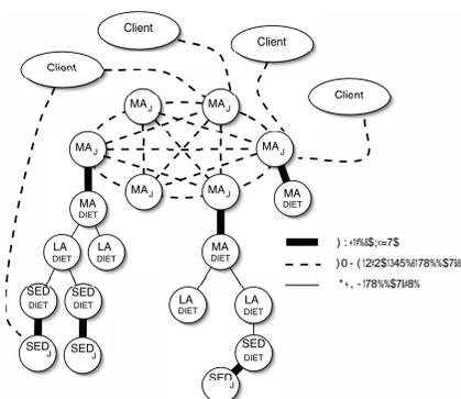
Figure 2: DIET<sub>J</sub> architecture.
