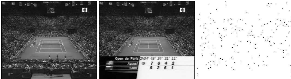
Figure 4: Robustness to occlusion. Despite the large occlusion the two images are detected as very similar with \log_{10}(NFA) = -50.1 . The right plot gives the position of the 200 sample points. There are not points in constant areas (because of the gradient threshold). However, some points are selected in the non-matching area (scores), but the NFA is still very low.
