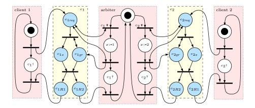
Figure 4: Petri net for the arbiter example
