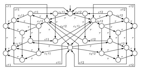
Figure 3: LTS for the arbiter example
