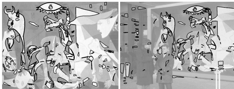
Figure 13: “Guernica” experiment: affine invariant meaningful matches [30]. Since all parallelograms differ from an affine transformation ( idem for triangles or ellipses), there are many casual matches.
