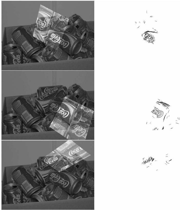
Figure 27: “Coca-Cola” experiment: registration with respect to the meaningful groups. Because there are several affine matches per group, one can compute the best projective mapping by a standard least squares method. The projective transformation is used to superpose the two images (on the left). On the right side, pieces of level lines that are close to each other in the registered images (see text).
